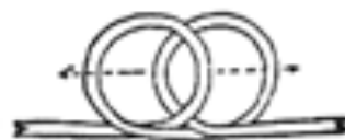
ROLLING HITCH is used instead of clove, and for guy lines.
